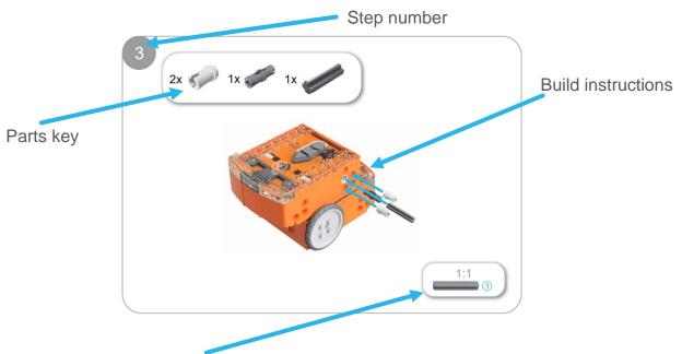
One-to-one piece measurement (when printed at 100% on A4 page). The number in the circle indicates the part's length in number of studs.
